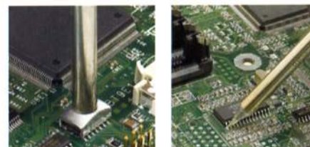
The Cartridge hand-piece uses small diameter cartridges for easy access and includes a full range for SMD rework.
