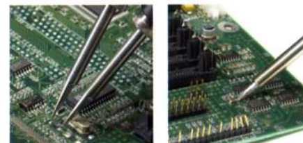
Precision Tweezers rework SMD components with fine dimension to large blade geometries, while the Soldering Tip hand-piece has exceptional power for production soldering.
